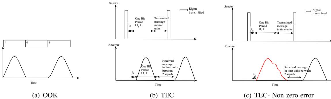
Fig. 3: Illustration of modulation schemes
