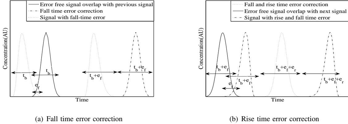
Fig. 5: Illustration of rise and fall time error correction
